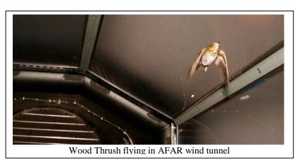
tunnel into which birds can be placed and their migration can be studied under a wide variety of conditions by changing air pressure (="altitude," up to 7000m), relative humidity (mimicking migrations over deserts/oceans, etc.), temperatures (-15C to +30C) and wind speeds. This equipment is complemented by use of quantitative magnetic resonance (QMR). This technique can measure within a 2 minute
